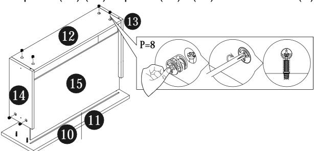
STEP 8-3:Fix rails (N-2) to panel (13) (14) with screw (V1)
